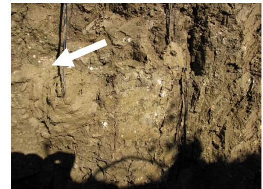
Costa Cavlieri station: shrinkage/swelling processes required initial period in which sensors had to progressively adhere to the surrounding soil after installation
