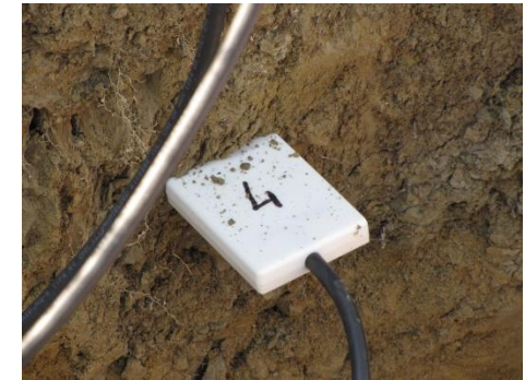
Montu  station: required initial period in which sensors had to progressively adhere to the surrounding soil after installation
