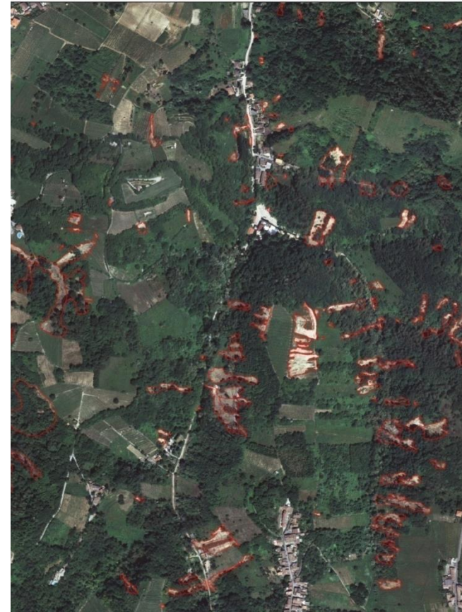
27 th -28 th April 2009 Event in Oltrepò Pavese (1639 shallow landslides in about 250 km 2 )
